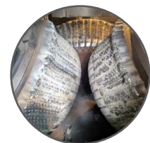
VRM-Sinter cast Liners Insitu after buttoning
