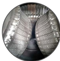
Sinter Cast Liners at 3000 Hours
