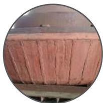
New Sinter Cast Liner in the VRM
