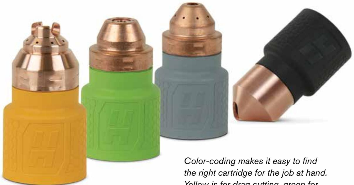
*Color-coding makes it easy to find the right cartridge for the job at hand. Yellow is for drag cutting, green for gouging, gray for mechanized cutting, and black for flush cutting.*
